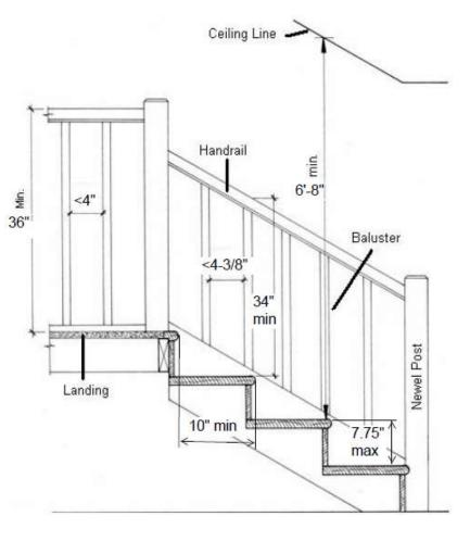
4. Guards shall not be less than 36" in height where the walking surface is located more than 30" above the floor or grade below, except that guards along the open side of stairs shall not be less than 34" in height measured vertically from the nosing of the treads. Guards shall be securely anchored to the structure to resist both vertical and lateral forces.
